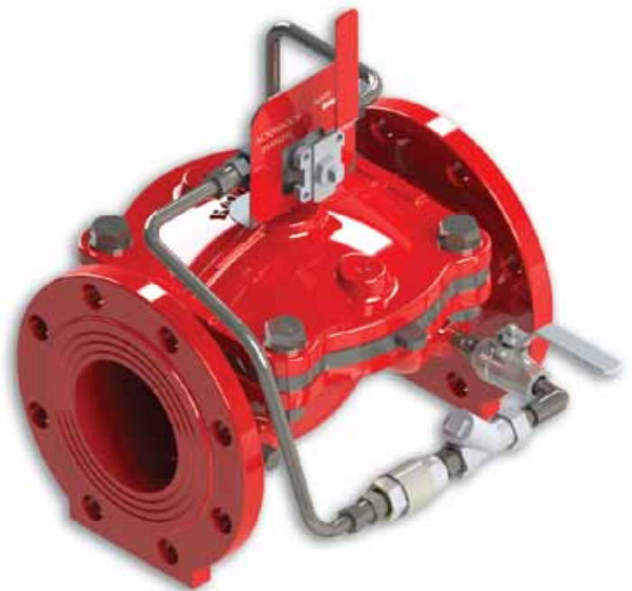
RAF-FP manual hydraulic actuation: Pressurize or vent control chamber to close or open RAF-FP Valve
